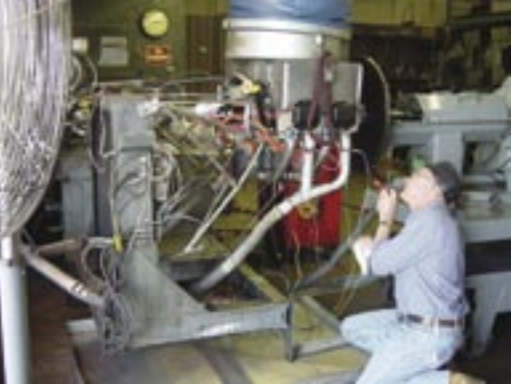
Post-run inspection revealed the engine to be leak-free.
